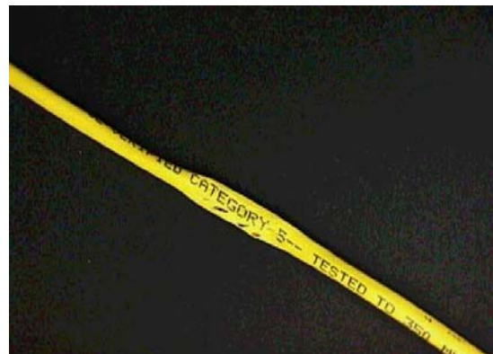
Photo 11: A cable that has been smashed or crushed. Note the cuts in the outer cable jacket
